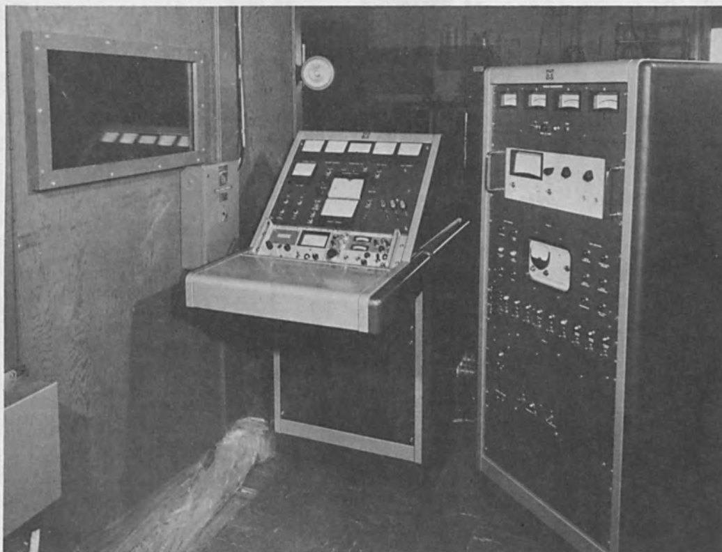
Figure 2. Side View of Installation for Nonvacuum Welder Showing Control Consoles.
