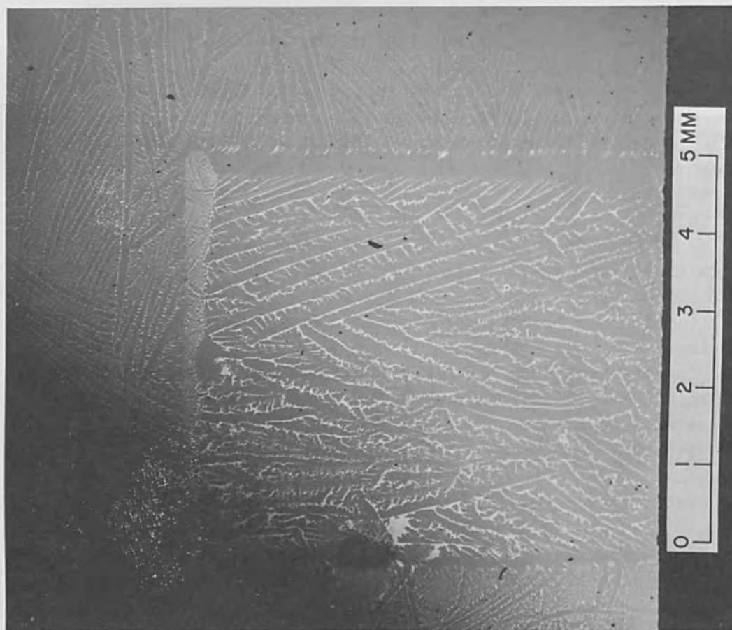
Figure 2b. Observe View of Same Film as Figure 2a, Taken Through Glass Substrate. Improved Ordering and Size of Dendrites are Apparent As Delineated by Metallic In Filaments.
