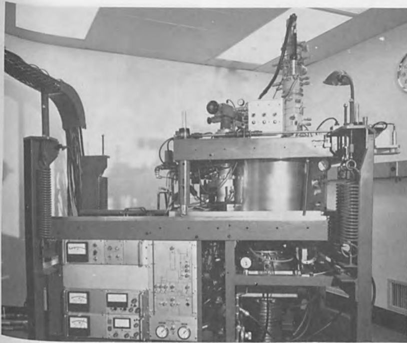
Fig. 3. Side view of the recorder with vacuum chamber closed and the column in the recording position.
