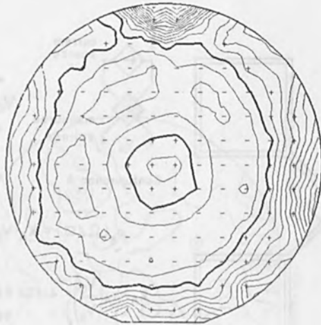
Figure 1 A sheet resistance contour map of a boron-implanted wafer obtained from a magnetic scanning implantation system.
