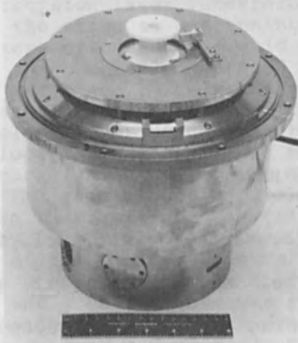
Figure 2. LWD Lens With Post-Lens Deflection Coil In Rotary Mount.
