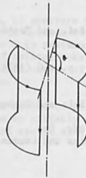
Fig. 5 - Form of deflection coil windings
