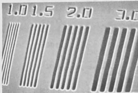
(b) Line patterns wet-etched in \text{SiO}_2 . Each figure shows line width in \mu\text{m} Thickness : 0.52 \mu\text{m} Etchant : buffered HF solution.
