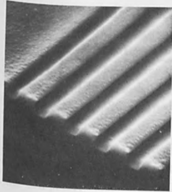
Fig. 7. Electronmicrograph showing the end profile of relief pattern in 1.1 \mu\text{m} of PMMA produced by x-ray lithography. The pattern has a 2.5 \mu\text{m} periodicity.
