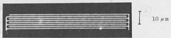
Fig. 7. A chromium mask for a surface wave transducer.
