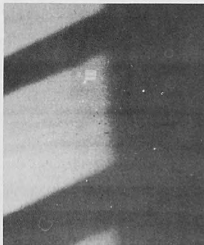
Fig. 1a. Argon ion bombardment of a gold film on a silicon substrate. (A) Shows the lattice of contamination lines laid down with the probe of the scanning electron microscope.
