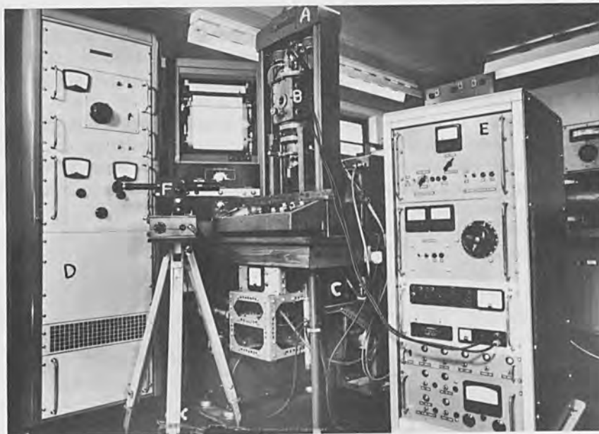
Fig. 3. (A) General view of tensile machine, (B) electron-beam furnace, (C) vacuum system, (D) power source, (E) control panel, (F) and optical pyrometer.
