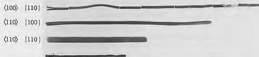
Fig. 2. Comparison of Mo-single crystals rolled down to 0.75-mm thickness with an as-grown crystal, 1:2,5.
