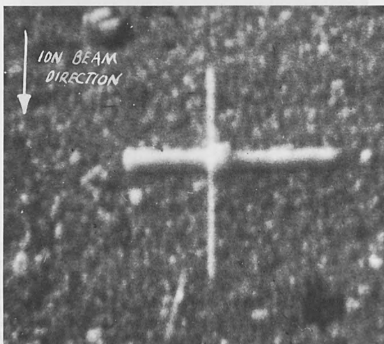
Fig. 3. A cross, micromachined by argon ion bombardment of a copper film.
