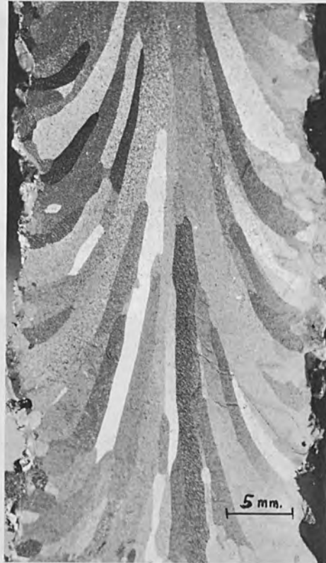
Fig. 8. Microstructures of electron-beam cast UC section parallel to the slug axis (columnar structure obtained for low casting rates).
