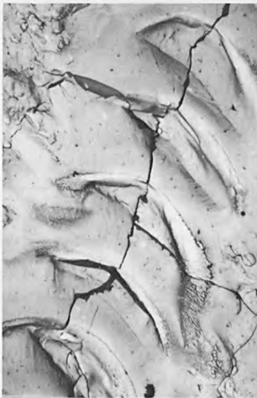
Fig. 4. An electron micrograph of a part of a groove cut by electron beam (accelerating voltage: 50 kV, ac heating).
