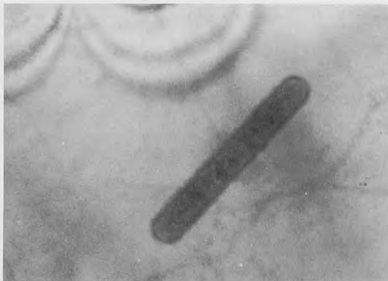
Fig. 8. Electron micrograph of precipitate in slowly grown crystal. Specimen from set B; zone speed was 0.2 mm/min. Surface shown is a \{100\} plane of a crystal of \langle 112 \rangle axial orientation. 100,000X.
