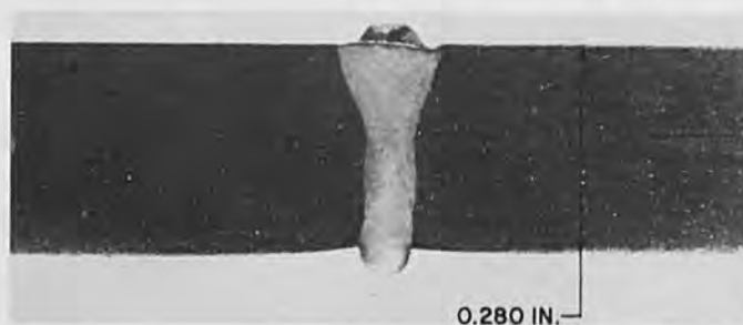
Fig. 2. Nonvacuum electron-beam butt weld—AISI 302 stainless steel.
