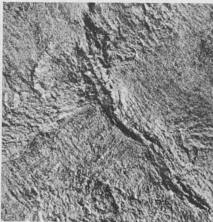
Fig. 13. Severe damage to tungsten by 60-cps oscillating beam at 3000°C for 15 minutes showing metal extruded up adjacent to grain boundary. X20.
