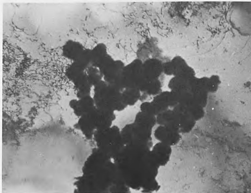
Fig. 7. Electron micrograph of precipitate in rapidly grown crystal. Specimen from set A; zone speed was 5 mm/min. Surface shown is a \{111\} plane of a crystal of \langle 111 \rangle axial orientation. 32,000X.
