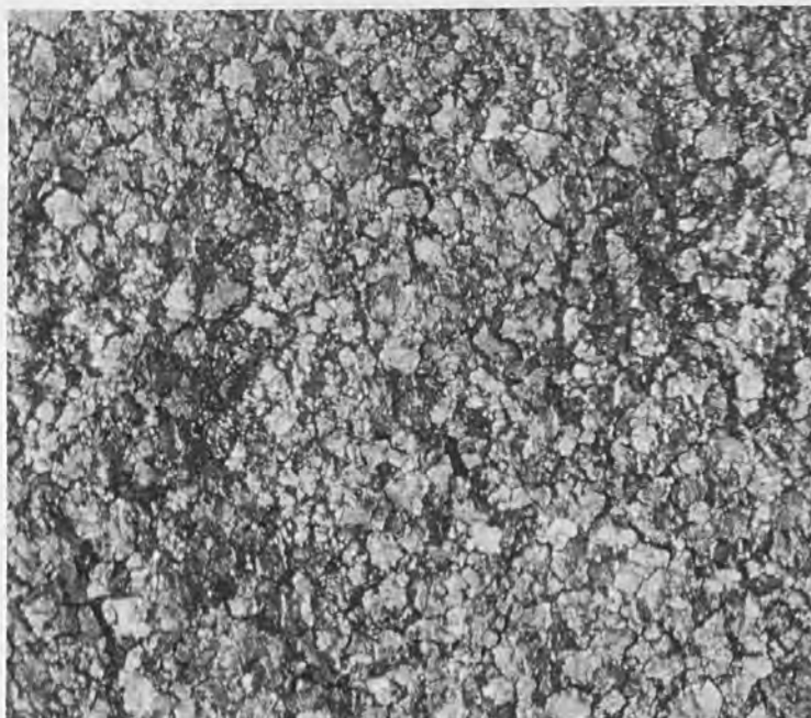
Fig. 12. Surface of polycrystalline sample damaged by 60-cps oscillating beam at 2600^{\circ}\text{C} for 30 minutes showing tilted and dislodged grains. X35.
