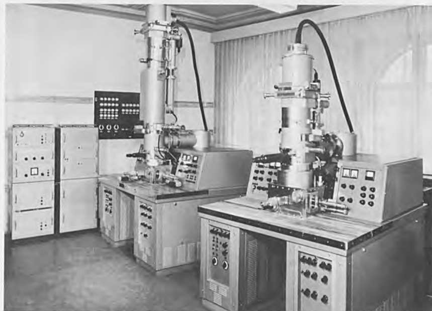
Fig. 7. View of one of the laboratories for electron beam tools with a 150-kV electron microprobe equipment (front) and an electron-optical 150 kV for micromachining of work pieces.
