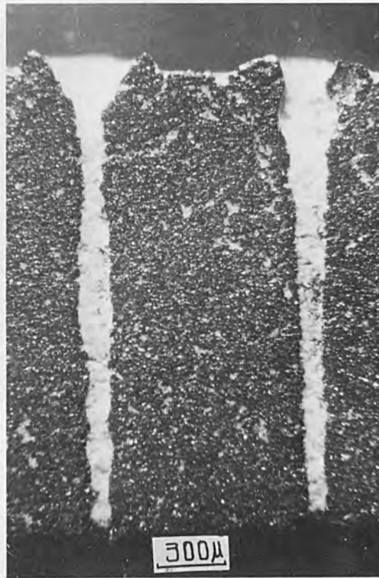
Fig. 11. Electron-beam perforation in 2-mm thick ferrite.
