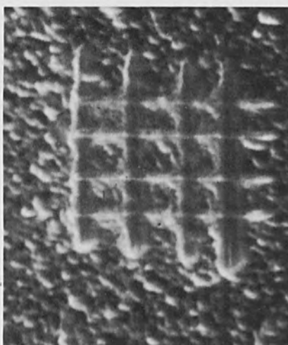
Fig. 1a. Argon ion bombardment of a gold film on a silicon substrate. (A) Shows the lattice of contamination lines laid down with the probe of the scanning electron microscope.
