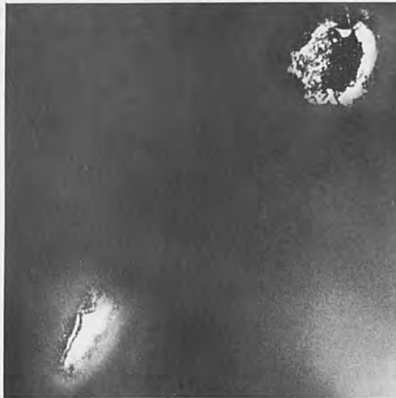
Fig. 3. Blister formation by subsurface heating (Brasch and Lange [3]).
