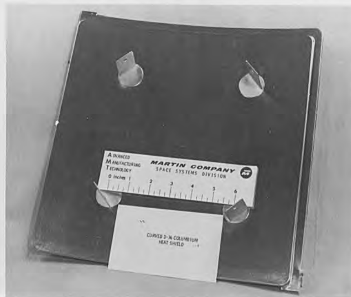
Fig. 2. D-36 brazed honeycomb heat shield panel.
