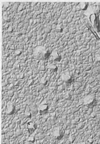
Fig. 10. Photograph of Al surface which is deposited on glass substrate by a narrow-shaped electron beam, 20,000X.
