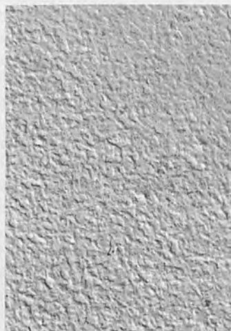
Fig. 11. Photograph of Al surface which is deposited on glass substrate by a wide-shaped electron beam. Power of electron beam is the same as Fig. 10, 20,000X.
