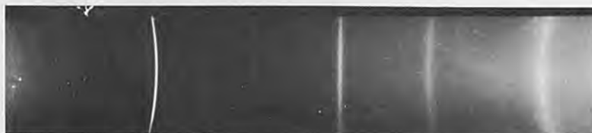
Fig. 4. A Debye-Scherrer x-ray pattern for a Ti-Co specimen containing 51.67 at % Co.
