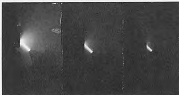
Fig. 52. Backscatter made visible in an atmosphere of 1 torr N_2 ; electron beam of 45 keV, 60 \mu A ; target: C (top), Al (middle), Pb (bottom) [85].
