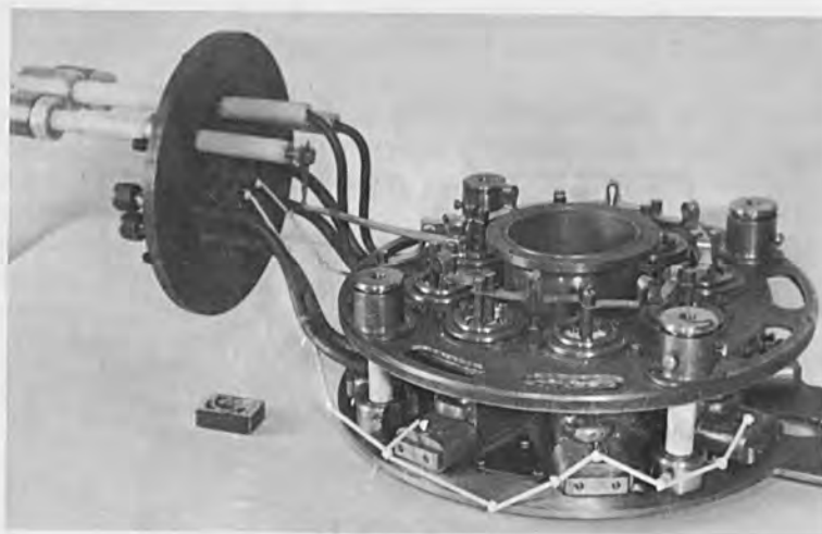
Fig. 4. General view of the electron-beam radial heater for melting of metals, power 150 kW.
