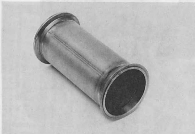
Fig. 11. Electron-beam welded experimental pipe for the bleed air piping of the VTOL-fighter VAK 191 B. Material: Ti-5Al-2,5Sn, wall thickness: 0.8 mm, pipe diameter: 115 mm. (Photo: VFW-Fokker)
