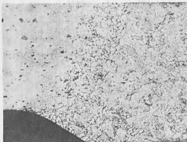
Fig. 7. Narrow-bead weld that exhibited high tensile strength
