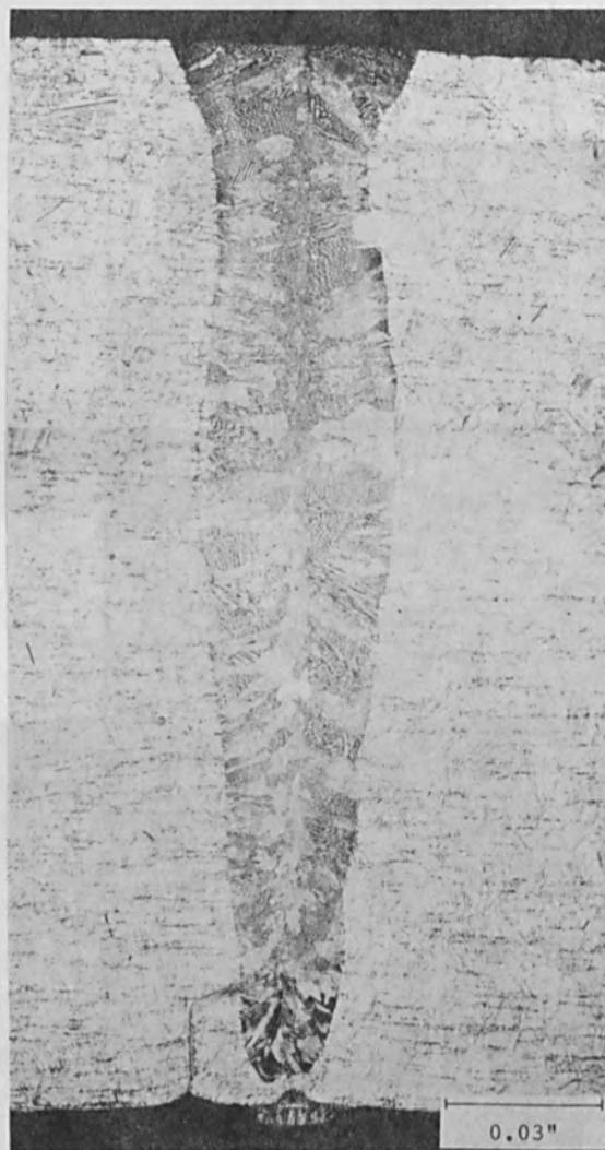
Fig. 20. EB weld in L605 phase II secondary cladding showing optimized penetration.
