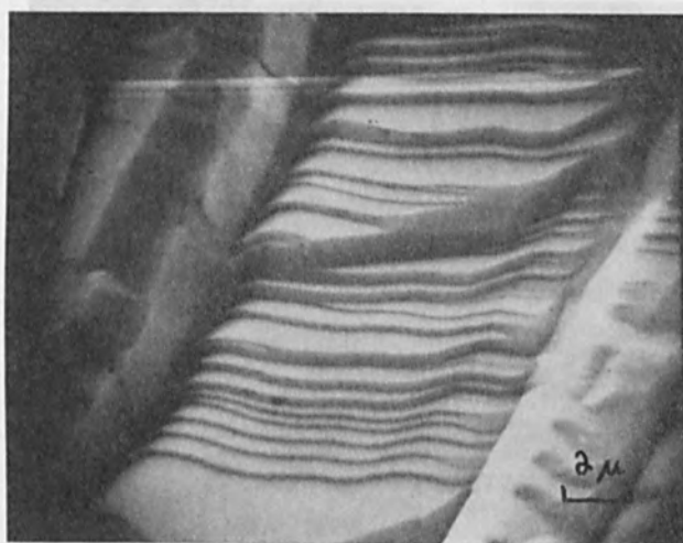
Figure 6. Coarse ledges observed in zinc.
