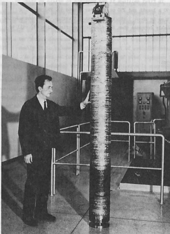
Photo No. 9. Refined Titanium Ingot ( \varnothing = 250 mm, l = 2.500 mm) in a 385 kW Power Gun.
