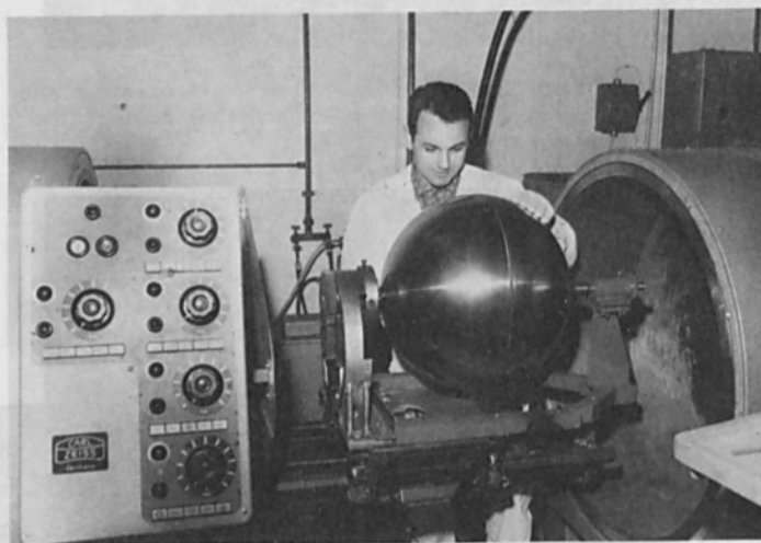
Fig. 17. Electron-beam welded satellite pressurized-gas tank for TD-2. Material: Ti-6Al-4V, wall thickness: 6 mm, diameter: 460 mm. (Photo: VFW-Fokker)
