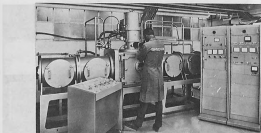
Fig. 8. Continuous bi-metal ribbon electron beam welding machine.
