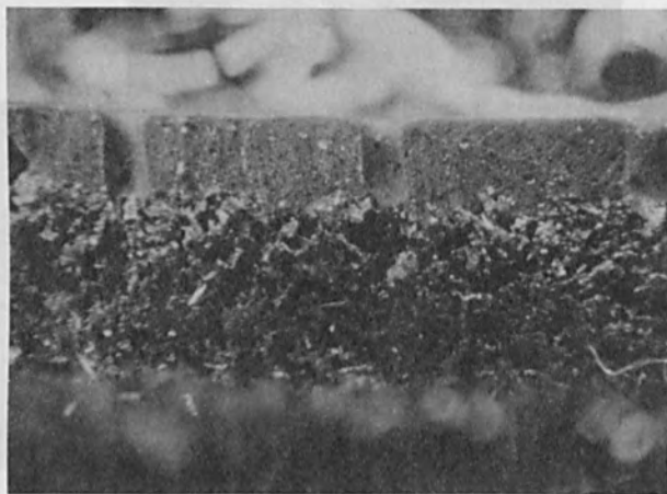
Fig. 14. Partially perforated artificial leather with holes of 170\ \mu diameter.
