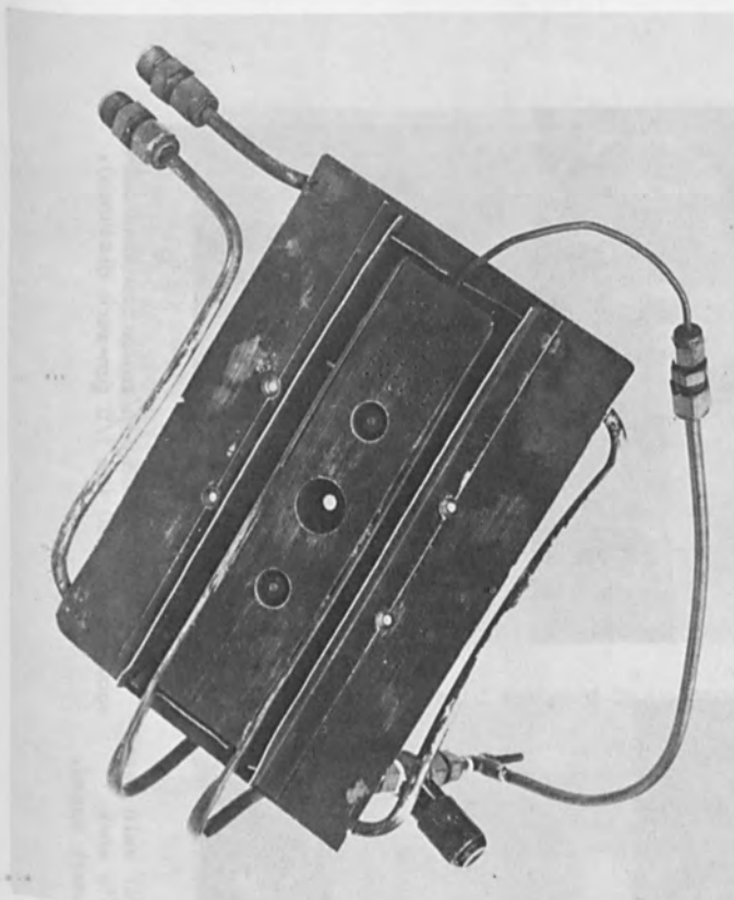
Fig. 3. Typical diffuser shield for providing inert gas coverage to the area around the point of beam impingement.
