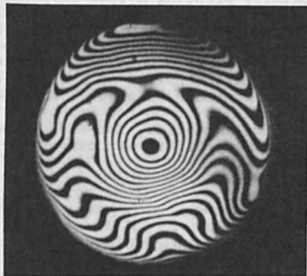
Fig. 5 Fifty seven mm diameter wafer showing non-flatness of wafer. Each fringe (bright to bright) corresponds to 0.32 micron.
