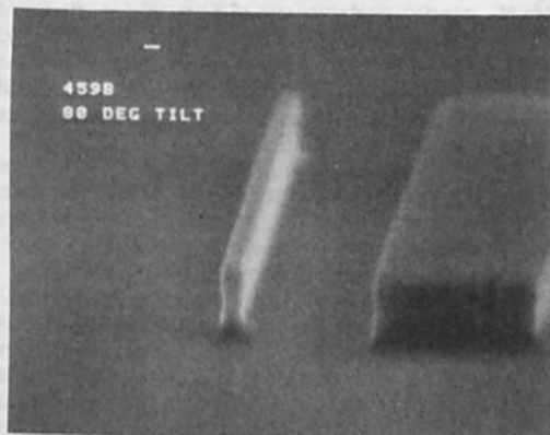
Fig. 4. An SEM photograph of a pedestal 100 nm wide by 300 nm high, formed by e-beam patterning and reactive ion etching into silicon.
