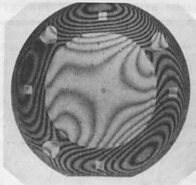
Fig.2 Photographs of flatness of a complex X-ray mask observed by an optical interferometer. Fringe interval corresponds to 0.27\mu\text{m} variation of flatness. Surface flatness is 3.3\mu\text{m} in the area of 2 inches in diameter.
