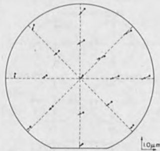
Figure 7. Overlay Performance using Titanium Mask. The arrows represent (to scale) the displacement vector at each location. The dashed lines are diameters with a common center. All the vectors lie in the lines indicating that the mask is stable, i.e. behaving as a rigid body.
