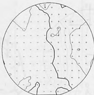
Fig. 9. Wafer implanted under conditions of unstable beam current.
