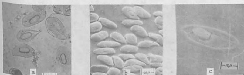
Fig. 6. Optical and electron micrographs of salamander blood cells stained with uranyl acetate. (a) is an optical photograph taken at normal incidence. (b) is an SEM micrograph of similar cells coated with a thin layer of aluminum and taken at a 60^\circ angle of incidence. (c) is an aluminum coated x-ray resist replica of the blood cells taken at a 60^\circ angle of incidence.
