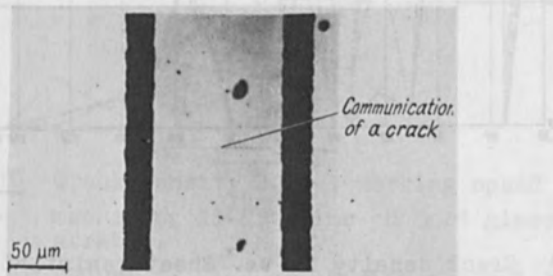
Fig. 8 Communication of a crack between adjacent tracks after thermal shock load. (Ni-Cr film on hard glass substrate, transmitted-light exposure).
