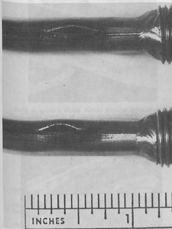
FIGURE 13 - NONVACUUM ELECTRON BEAM WELDMENTS IN 0.020" (0.5 cm) THIN WALL INCOLOY 800 TUBING WELDED AT 7.8 kW, 3/8" STANDOFF ( \sim 1 cm), 1200 IN./MIN. (51 cm/SEC) WITH AIR EFFLUENT. DUCTILE RUPTURE OCCURRED IN WELD SEAM AT INTERNAL PRESSURE OF 11,000 PSI.
