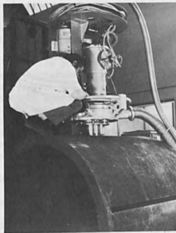
Fig. 3 : Electron gun for bore welding and test-piece. Fig. 4 : Portable E.B. welding machine for nozzles.
