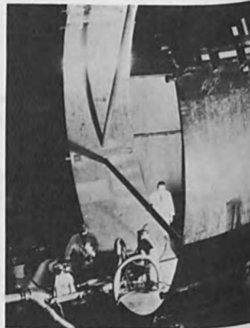
Fig. 6 : 6 m diameters shells E.B. welded by portable machine (doc.Neyrpic).
