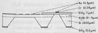
Fig. 8. Schematic cross section of a transistor fabricated using x-ray lithography. The emitter oxide cut also serves as the contact cut. Four lithographic steps were required, in three of which the mask pattern had to be registered with respect to previous patterns.
