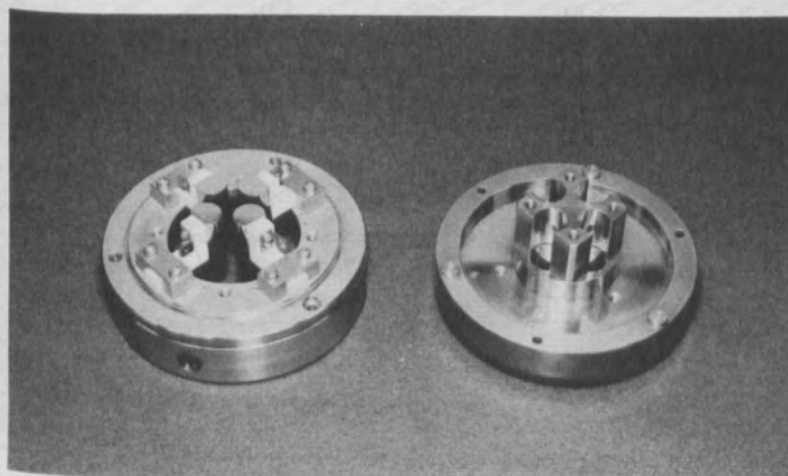
Fig. 4 Electrostatic quadrupole lens and alignment jig.
