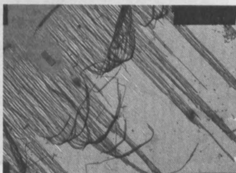
Fig.5(a) Boundary between solid & thin substrate exposures at 1.95E_c . Note that pattern quality is poor on thin film side of focusing square, presumably due to scattering out of the substrate.
