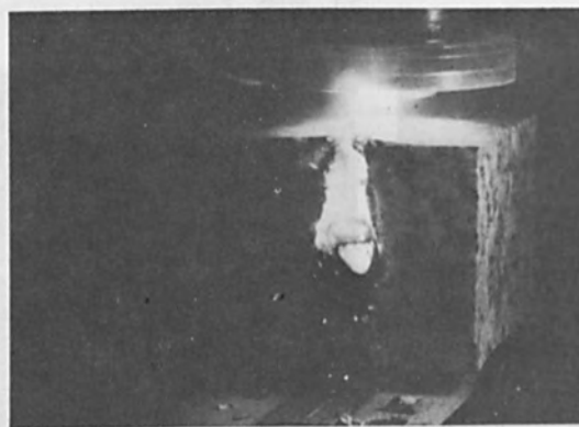
Fig. 4. Granite block moving into the electron beam; Top: Beam 3/4 " from front face of block; Middle: Beam 1/16 " from front face of block; Lower: Beam cutting slot into the solid rock.
