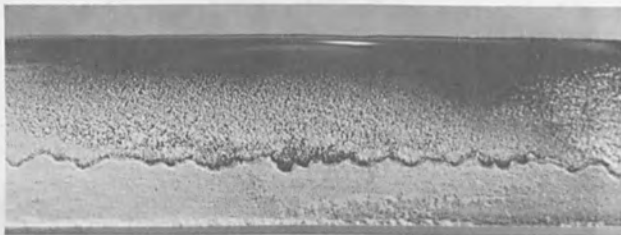
Figure 6. Penetration Pattern in Electron Beam Welded Uranium.
