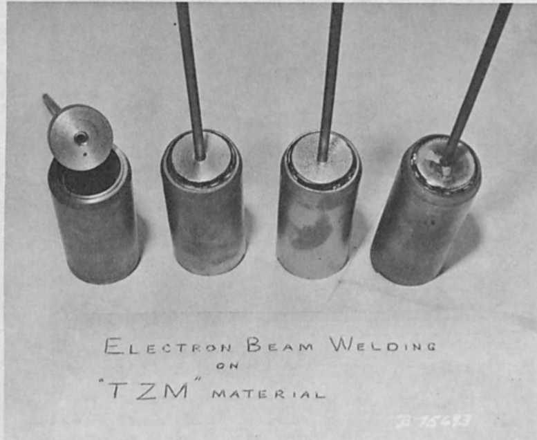
Figure 13. Fuel containers electron beam welded.
