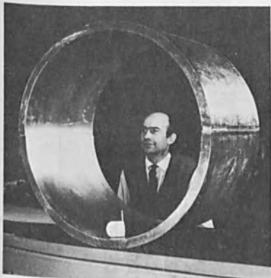
FIG. 1 : BUTT-WELDED 70 cm DIAMETER LINEAR ACCELERATOR COMPONENT
