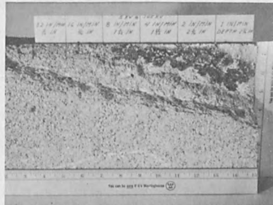
Fig. 11. E.B. cuts in concrete block; with 5 and 9 kW cutting speeds; Lower picture shows break of 5 kW cut.
