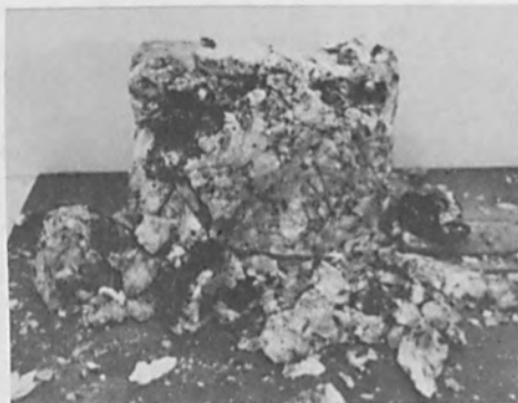
Fig. 8. E.B. cut of granite block producing thermal cracking.
