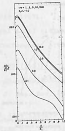
Fig. 8. Minority carrier concentration profiles for successive time steps.
