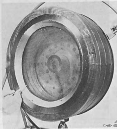
Figure 13. - Fused glass composite accelerator grid mounted on a 30 cm diameter Kaufman thruster.
