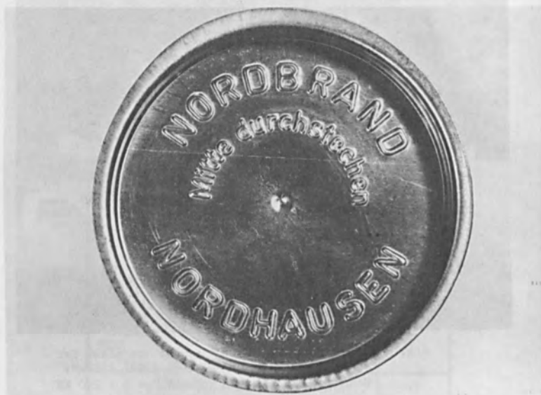
Fig. 9: Bottle lid with sharp coinings from aluminium vapor deposited steel strip. There occurs no burst off.
