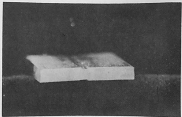
FIGURE 8 Butt weld: 1/8" thick stainless steel 108KV, 6 ma work current, 6ipm pass speed
