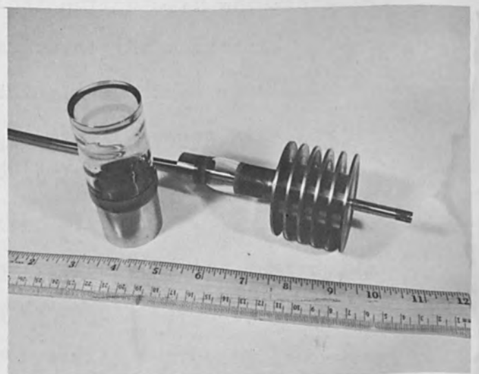
Figure 9. Viewport and High Voltage Terminal
