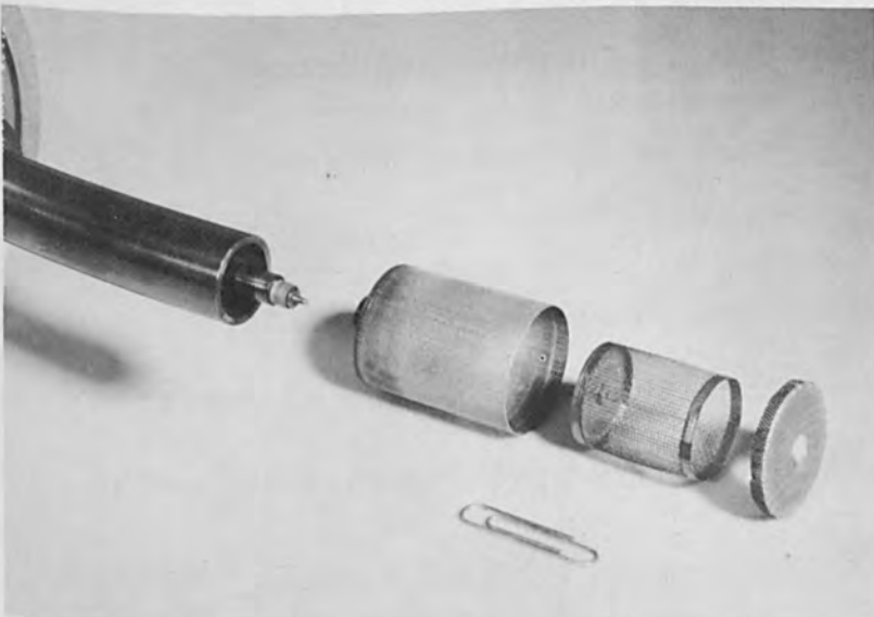
Fig. 6 EXPLODED VIEW OF GRID CONTROLLED CATHODE ASSEMBLY
