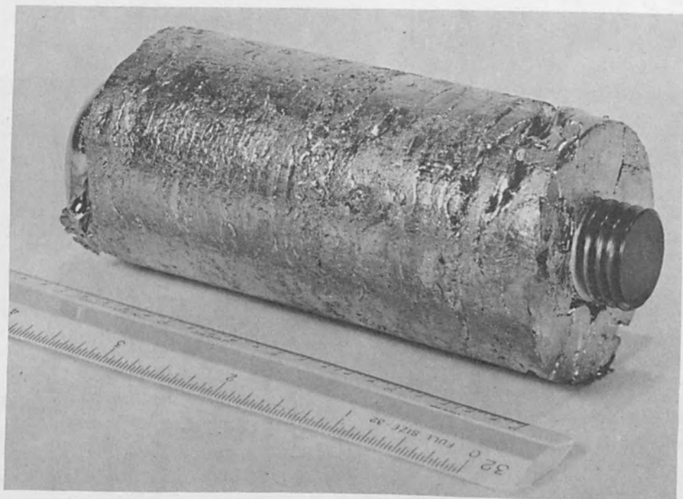
Figure 8 Titanium Ingot Melted by Electron Bombardment (2" dia.)
