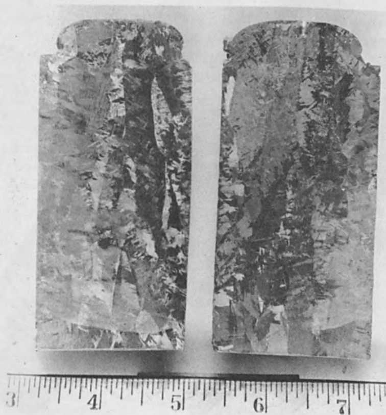
Figure 9 Sectioned Titanium Ingot
