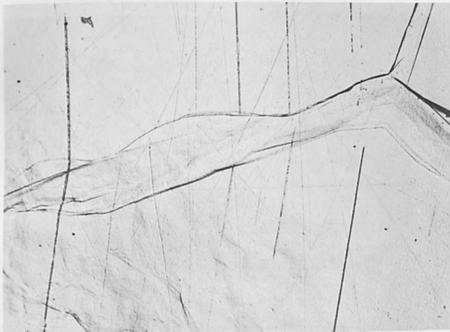
Fig. 9. Rotation of Adjacent Grains During Boundary Movement on Annealed Silicon Iron. (X150)
