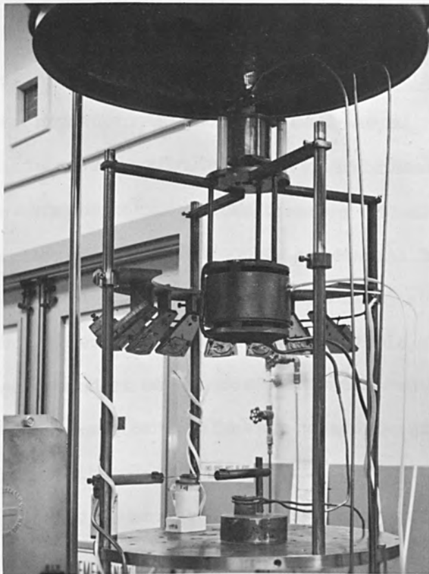
Figure 4 Vacuum System and Tooling used to Make Controlled Nichrome Resistor Films by Electron Beam Evaporation.
