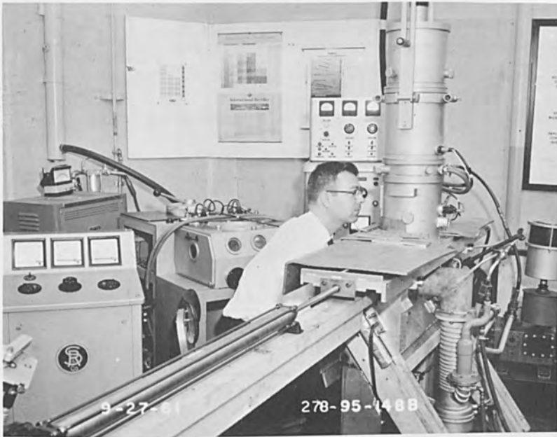
Figure 22. Prototype Portable Vacuum Chamber.
