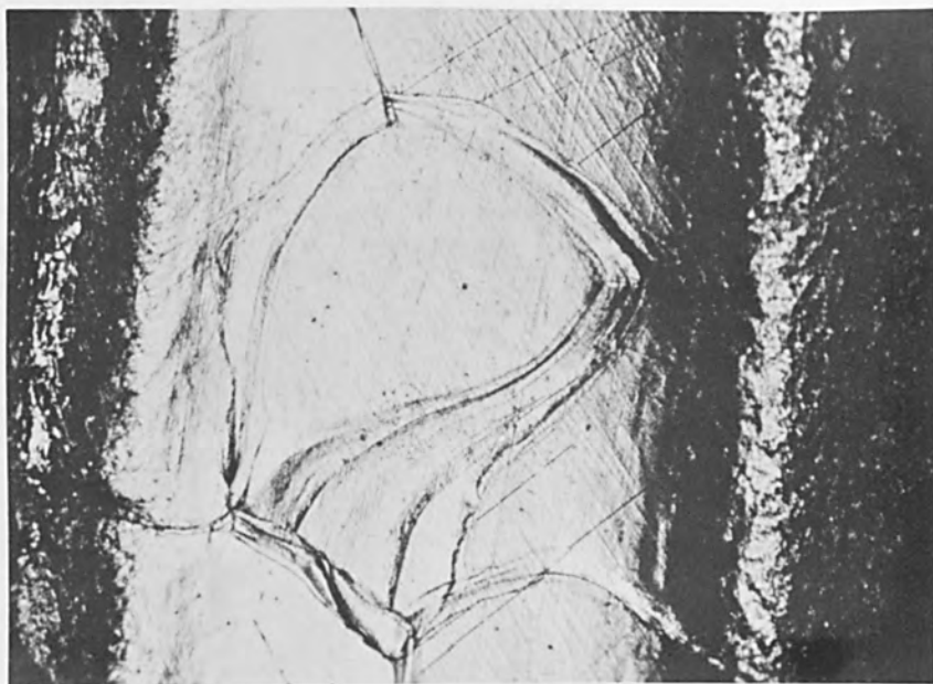
Fig. 7. Grain Boundary Migration on Annealed Silicon Iron Showing Progressive Positions During Movement. (X75)
