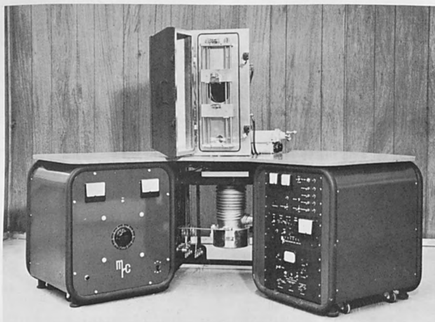
Figure 1. Electron Beam Floating Zone Apparatus
