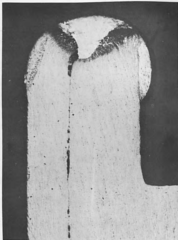
Fig.14. Type a - welding of S.A.P. 895 degassed. X25
