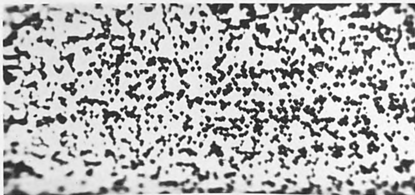
Figure 4. Etch Pits on Cube Face (100) of Tungsten Single Crystal Grown by Strain-Anneal Method. Axis of Crystal Within 3^\circ of [\bar{0}11] . Electrolytically Polished and Etched with 2% NaOH. (250X)
