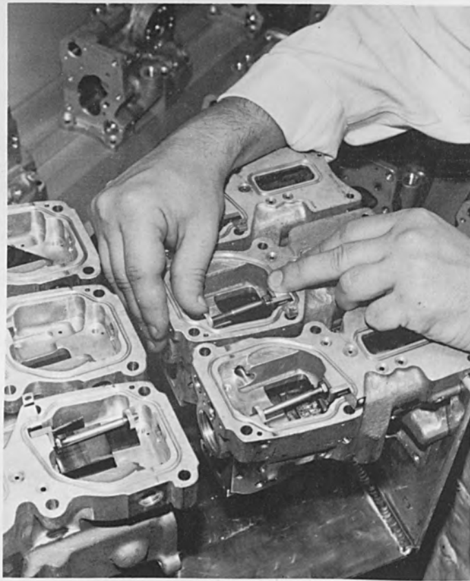
Figure 12: Fixturing of Castings for Repair Welding
