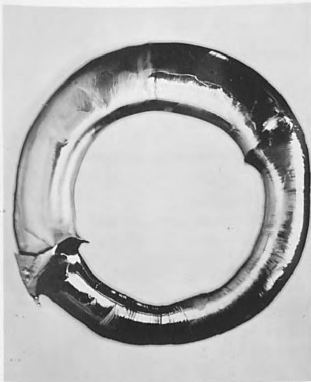
Fig. 2. Columbium Ring Zone Melted at \frac{1}{4} rph with a Shaped (Top) and Unshaped 17.6-kw Electron Beam.
