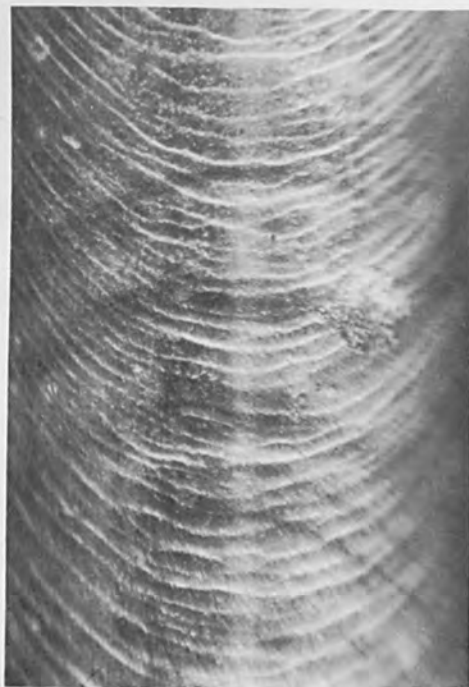
Fig. 16. Slip lines on a Tungsten single crystal
