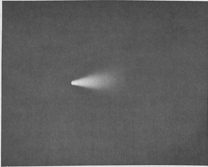
Figure 4 Photograph of electron beam entering atmosphere when N_2 protective gas is used.
