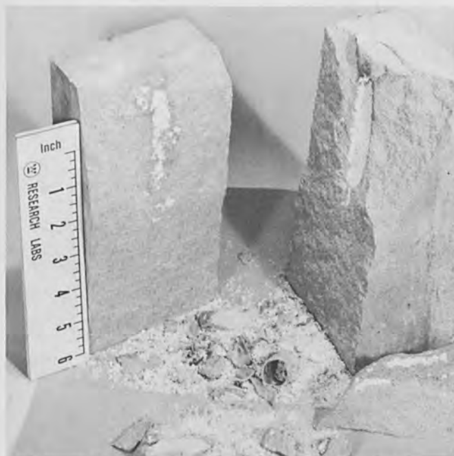
FIG. 11.—Limestone block pierced by a 9-kW electron beam in the direction of the long axis to prevent burning through without breaking; breakage occurred after 57 sec.
