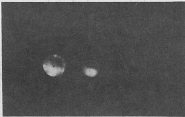
(b) Time-differentiated electron spatial distribution, 5 ns/frame, f/2 plus neutral-density filter \times 40 . (Time increases to right.)
