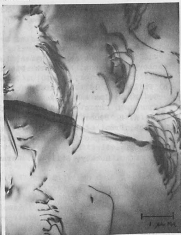
FIG. 10.—Dislocations associated with surface scratches on an alumina ( \text{Al}_2\text{O}_3 + \frac{1}{4}\% \text{MgO} ) specimen.
