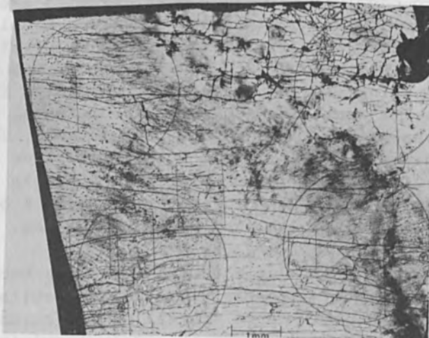
FIG. 3.—Petrographic thin section of Brazil quartz deformed under confining pressure.
