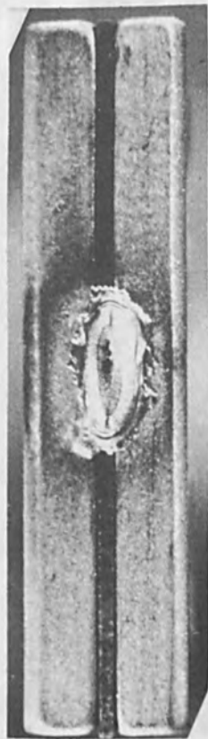
FIG. 4.—End view of the spring-leaf assembly showing the elliptical weld spot.
