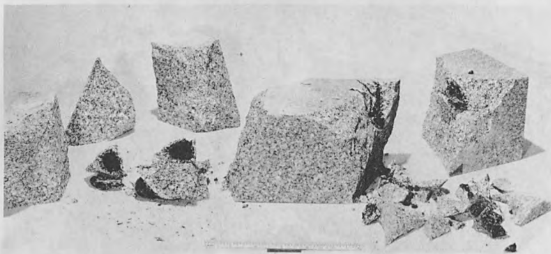
FIG. 7.—Fine grained granite from Vermont. On the left breakage induced by stationary 9-kW electron beam after 56 sec. On the right breakage induced after 57 sec by 9-kW beam traveling at 4 IPM. The melt-cavity broke away from the block as a separate tubular piece.
