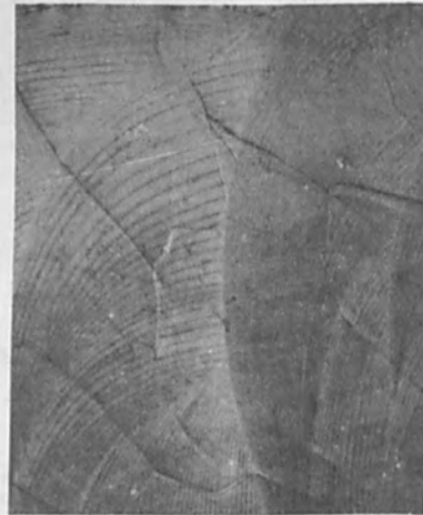
FIG. 4.—Laue back-reflection micrograph of columnar grained weld region.
