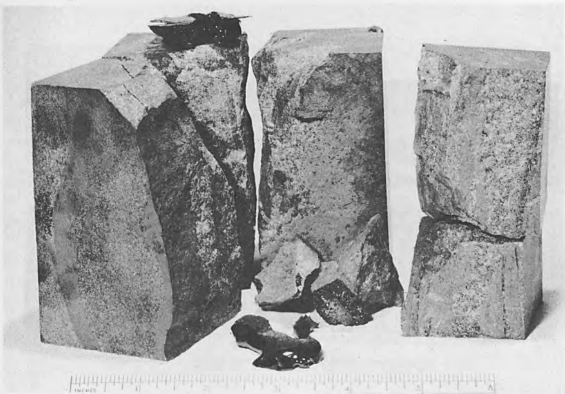
FIG. 5.—Reserve taconite, thermal-stress cracking produced by stationary electron beam.
