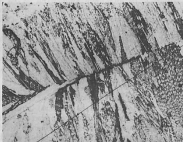
FIG. 5.—Shrinkage in FZ solidification center line in A-286. (Courtesy: J. Pasoja, Fusion Division of EBTEC.)
