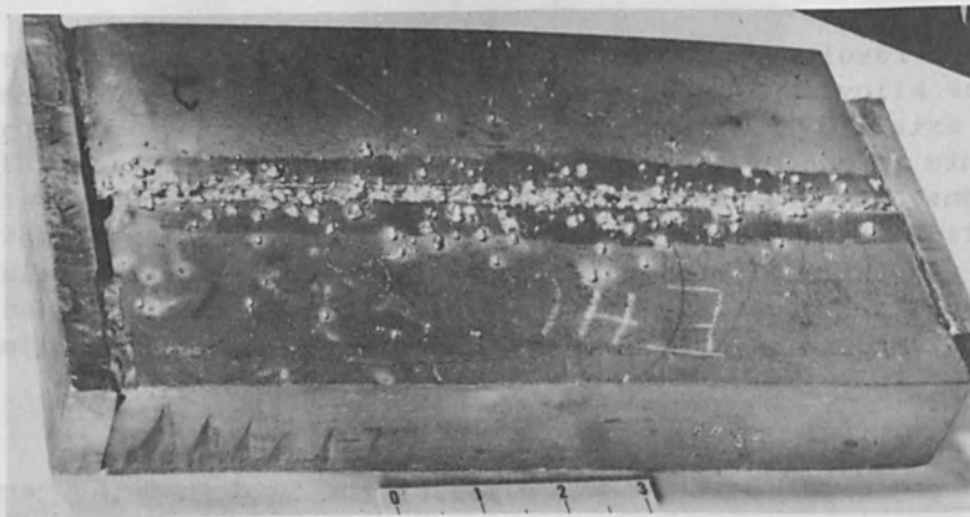
FIG. 4.—Spatter on surface of weld in 1.5-in. HP 9-4-25. (Courtesy: J. Gerken, TRW.)
