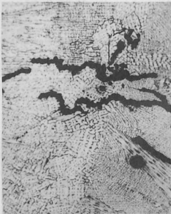
FIG. 6.—A-286 cracking in coarse grained structure. (Courtesy: J. Pasoja, Fusion Division of EBTEC.)
