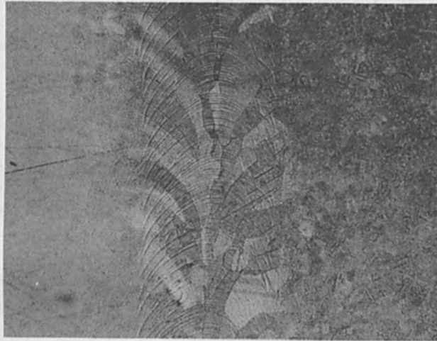
FIG. 2.—Photomicrograph showing scalloped edge of columnar grained EB weld region (mag. 100X).
