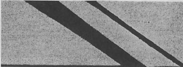
FIG. 6.—Oblique holes drilled in Ni alloy, 3.3 mm thick; hole length 5.2 mm, angle to surface 35^\circ , diameters 0.7 and 0.2 mm, drilling time 15 and 3 sec.
