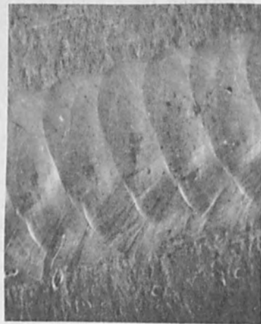
FIG. 4.—Laue back-reflection micrograph of columnar grained weld region.
