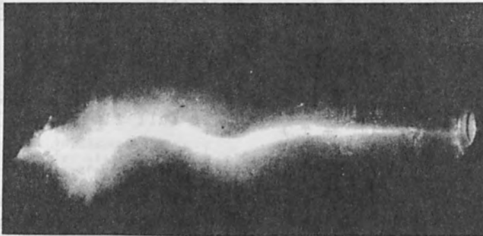
FIG. 8.--"Frozen hose" instability of a pinched beam. Instability wavelength is \sim 16 cm. Beam parameters: pressure 0.1 torr; beam current \sim 25 kA; average kinetic energy \sim 3 MeV; current risetime \sim 10 ns. Beam is traveling from right to left.
