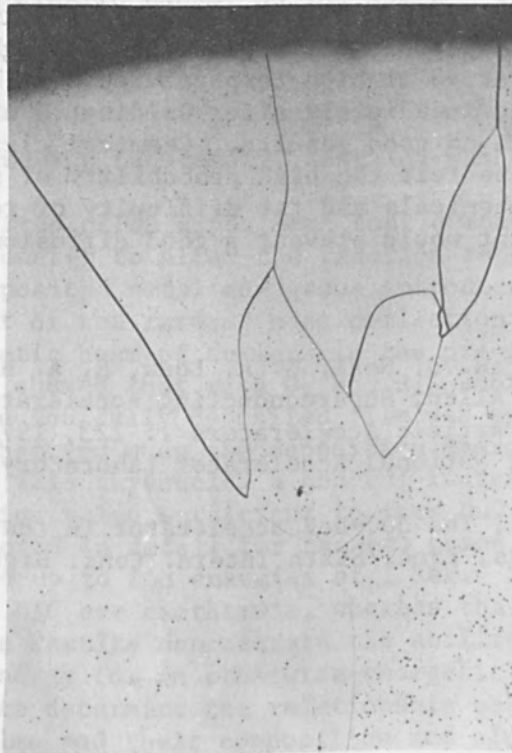
FIG. 9.--Electron-beam weld in niobium after vacuum annealing at 2000°C for 20 hr (50 x).
