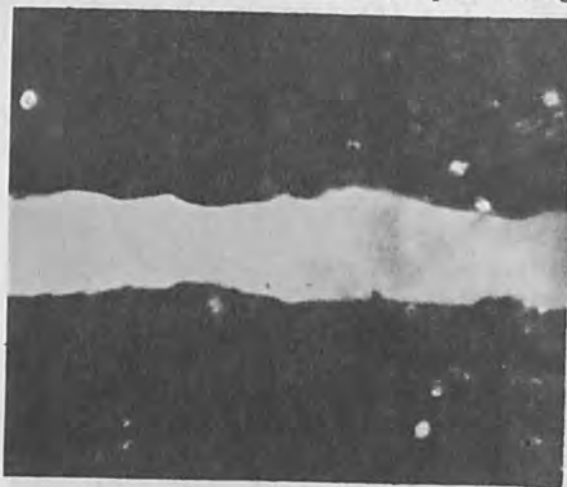
FIG. 8.--Cutting through 2-mil stainless steel with an argon laser.
