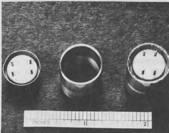
FIG. 6.--Kovar thermocouple gage header, co-extruded transition cylinder, and laser-welded sub-assembly.
