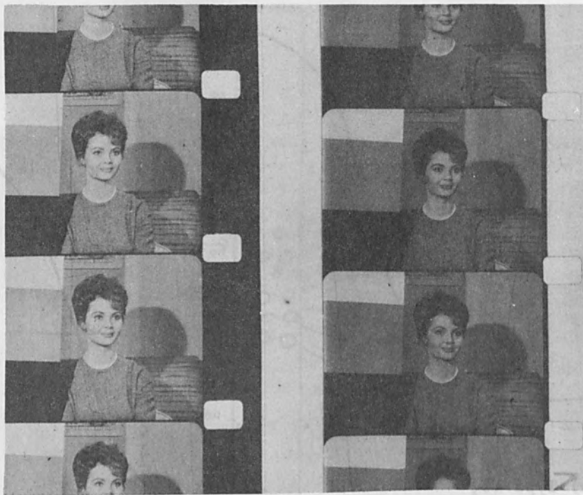
FIG. 5.--Release Prints: Kalvar Type 23 (left) and Silver halide cine positive of same negative.
