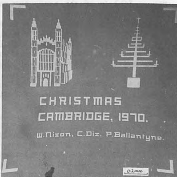
FIG. 4.--Christmas Card etched in silicon dioxide on silicon using electron-beam-exposed resist. Note complexity available within a 10^3 \times 10^3 matrix. (Optical micrographs.)
