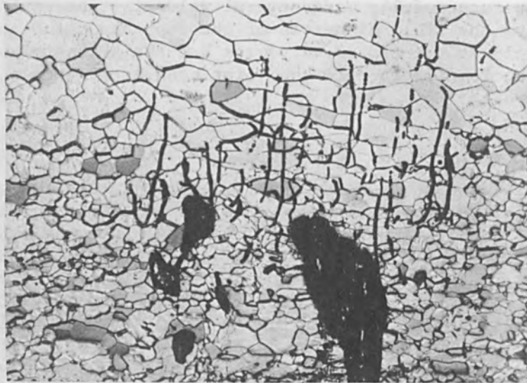
FIG. 7.--Cold shuts in electron-beam welded niobium. Weld is at top and parent metal at bottom; weld direction to right (50 x).
