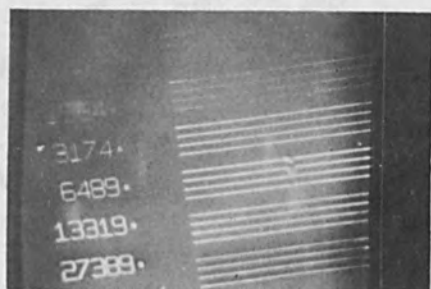
FIG. 8.--Scanning electron micrograph of exposed lines and numbers on plastic block sample.
