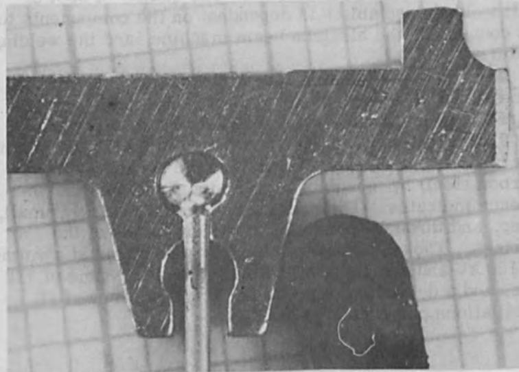
Figure 2. Electron beam spot weld of hammer and leaf spring (top view).
