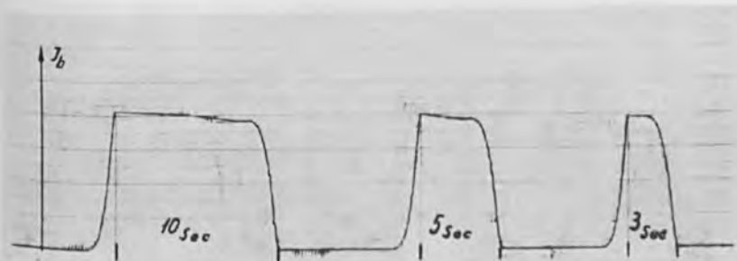
Figure 11. Form of long current pulses of different durations.
