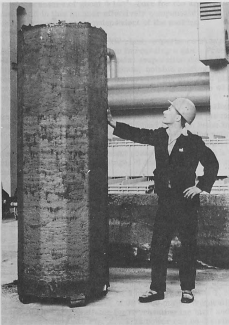
Figure 6. Metal ingot, having been remelted in the 1,700 kW multichamber electron beam furnace of VEB LEW/GDR. P = 1200 \text{ kW} e = 1.5 \text{ kWh kg}^{-1} G = 8000 \text{ kp}
