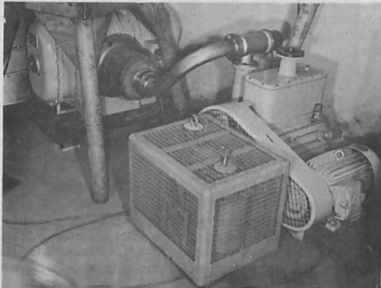
Figure 1. Rotary-valve and Root's pump of the ZIS 456 electron-beam welding unit.
