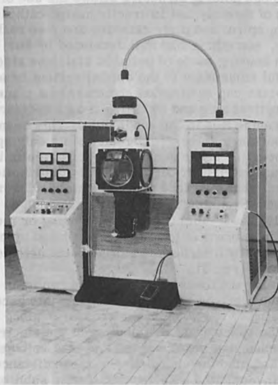
Figure 2. The 2 kW, 25 kV electron beam welding machine Type ESH-21, developed for use in the instrument industry.
