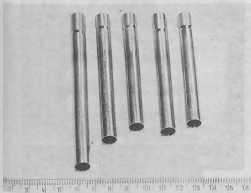
Figure 9. Welded-in plugs on nuclear fuel elements.
