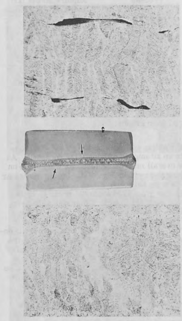
Figure 4. (a) Macrostructure of Two Pass Weld in 1.5 Inch Ti-6Al-4V. Made on 30 kW Electron Beam Welder. (b) Tip of Fusion Zone of Second Pass Showing Absence of Cold Shut. (c) Cold Shut Occurring Along Walls of Fusion Zone (HF + HNO 3 + H 2 O Etch). Weld Parameters - 50 kV, 320 mA, 65 ipm
