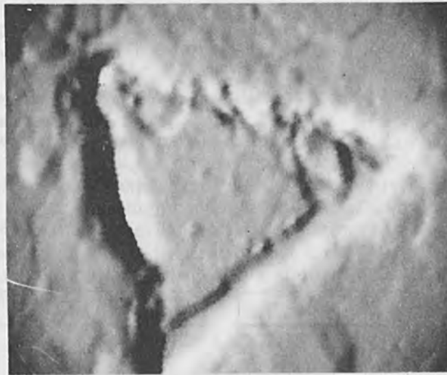
Figure 13. Differentiated Electron Beam Induced Current Display (EBIC) Simulates Exactly the EBITC Display Shown Above Beam Voltage = 18 kv M = 12,000x Scan Time = 64 ms/Line, Rc = 10^{-4} Sec.
