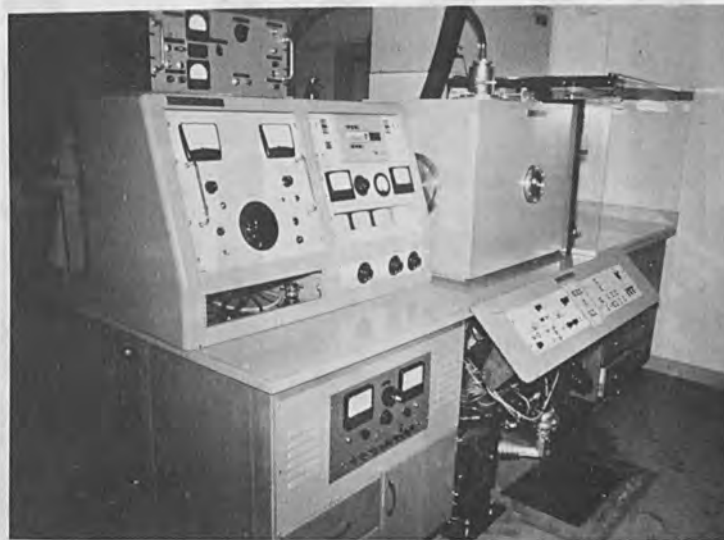
Figure 6. Implantation Equipment for Solar Cell Production (Ion Physics Corporation).
