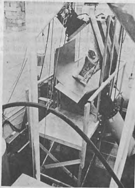
Figure 4. Arrangement for Surface Pasteurization of Beef Quarters Using Two 300 Kev Electron Irradiators. Beef Quarter Rotates During Passage Between the Beams. (High Voltage Engineering Corporation).
