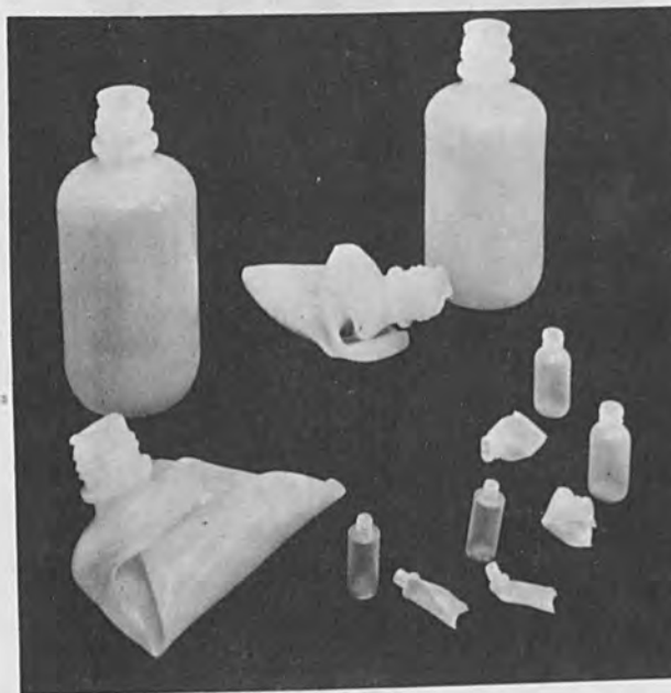
Figure 3. Irradiated Polyethylene Bottles and Controls After Heating. Unirradiated Controls have Collapsed. (High Voltage Engineering Corporation).
