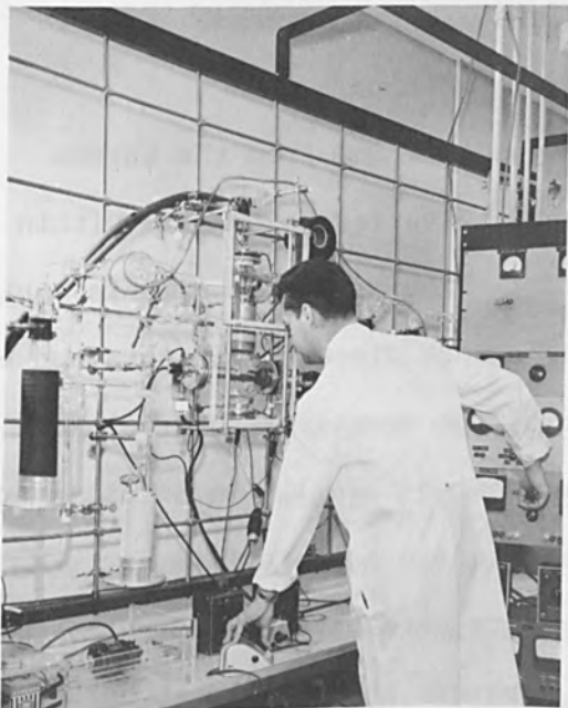
FIGURE 1 Differentially Pumped Electron Beam System
