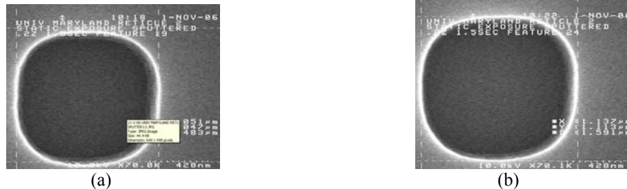
Figure 3: SEM image of resolved pattern with X and Y measurement; a) pattern 19; b) pattern 24
