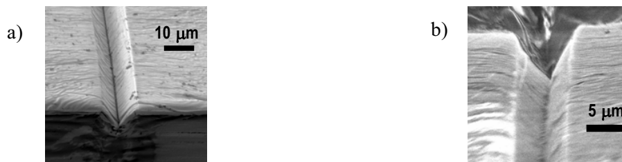
Figure 4. SEM images of the final structures in gold (scheme in figure 1, f), using the oxidized stamp shown in figure 3. The shape has been improved, as can be seen in (a), and especially in (b).
