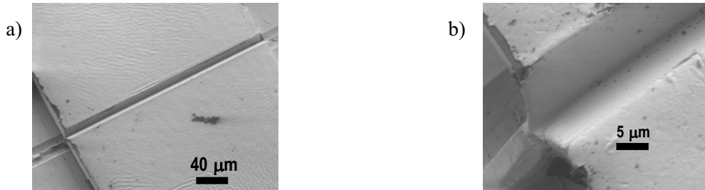
Figure 2. SEM images of the final structures fabricated in gold (figure 1 f). (a), the groove and the deep channels. (b) a detail of the v-groove, showing the smoothness of the sidewalls.
