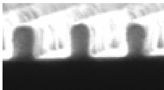
Figure 2: Cross section of 100 nm pitch dense lines printed with EUV-IL.
