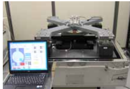
Fig. 3. Photograph of our nanoimprinter.
