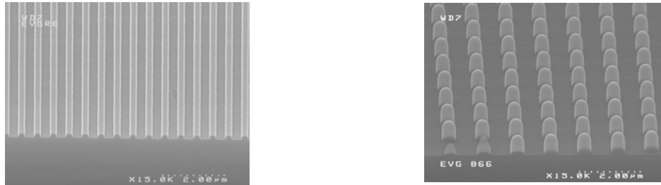
Figure 1: 240/260 nm lines and 440 nm wide, 650 nm high pillars imprinted in the NEB22 resist
