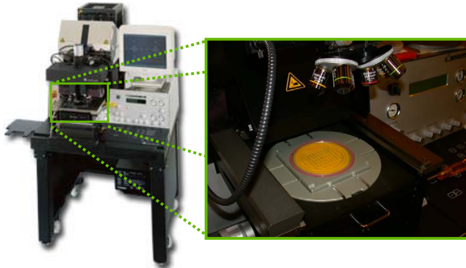
Figure 1. With the nanoimprint module loaded, a contact mask aligner is transformed into a nanoimprint machine.
