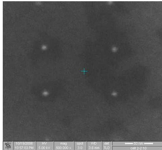
Figure 1 6 nm dots (with 125 nm pitch in the x direction and 100 nm pitch in the y direction) written in a 20 nm HSQ layer; the area dose is 586731 \mu\text{C}/\text{cm}^2
