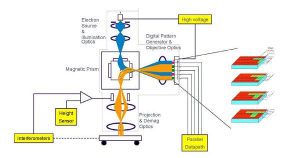
*Fig 1:* REBL system schematic showing the reflective electron optics configuration. The Electron Source illuminates the Digital Pattern Generator (DPG) through the Magnetic Prism. The reflected electrons from the DPG, which define the pattern to be exposed, pass through the Magnetic Prism again, which separates them from the Illumination Beam. The DPG image is then demagnified and projected onto the wafer.
