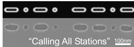
Figure 3. Morse code pattern "CQ" printed by nanostepping a single mask feature (~30 nm) 28 times demonstrates the exceptional precision and accuracy of the nanostepping process 2 .
