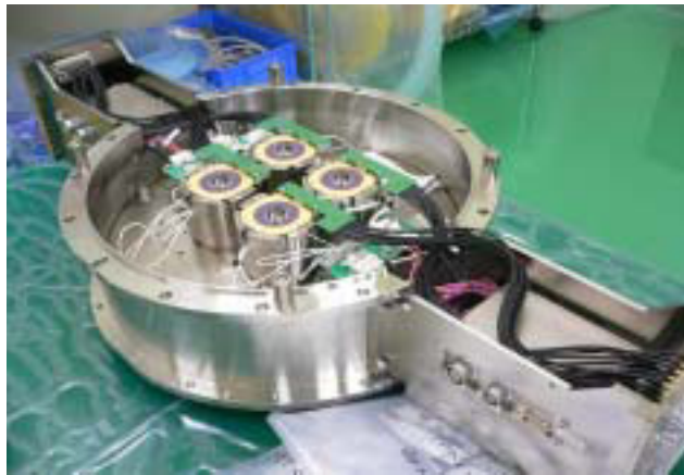
Figure 1. A lens unit of the MCC column in the POC system. The lens unit has four electromagnetic lenses in a permalloy frame. Each lens diameter is less than 70mm.
