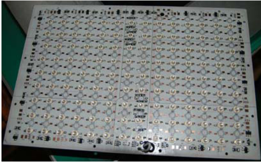
Fig. 2. Photograph of the UV-LED array(14 x 9) lamp.
