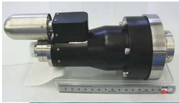
Fig.1 Photographs of the developed low-energy soft X-ray CT system installation, and the X-ray tube for the low-energy soft X-ray generation.
