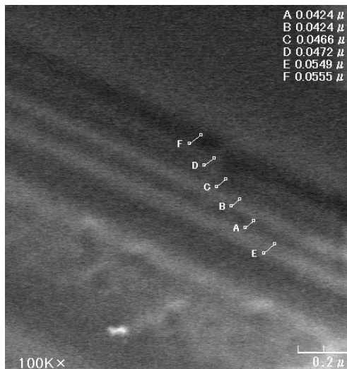
Figure 2. SEM Image of approximately 40nm-wide Line & Space pattern exposed on EB resist of the target.
