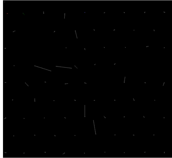
Fig 2. Force field from an axonal growth cone. The magnitudes and directions of the forces generated by the evolving structure are illustrated. The distance between wires (horizontally) is 1 \mu\text{m} .
