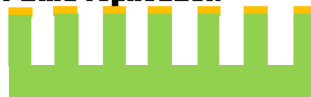
Figure 1. Schematic drawing of the fabrication of PDMS pillars with gold layer on the top.
