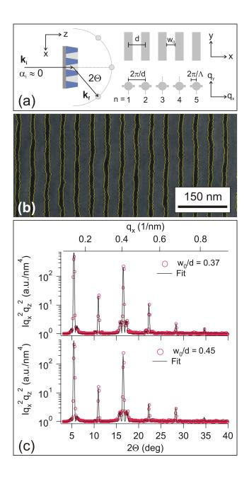
Fig. 1: (a) Illustration of diffraction geometry, and dimensions of the epitaxial template/block copolymer resist. (b) Scanning electron microscopy measurement of the lamellar block copolymer resist. Edge positions are highlighted in yellow. (c) Diffraction data from block copolymer resists assembled on epitaxial templates with duty cycles  $w_0/d \simeq 0.37$  and 0.45. Solid lines are the best-fit results.
