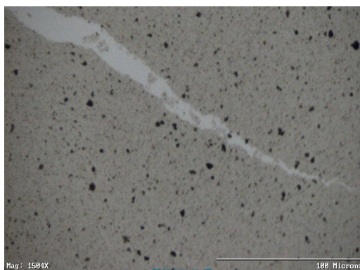
Figure 2: A (scratched) monolayer thick layer of ruthenium oxide
