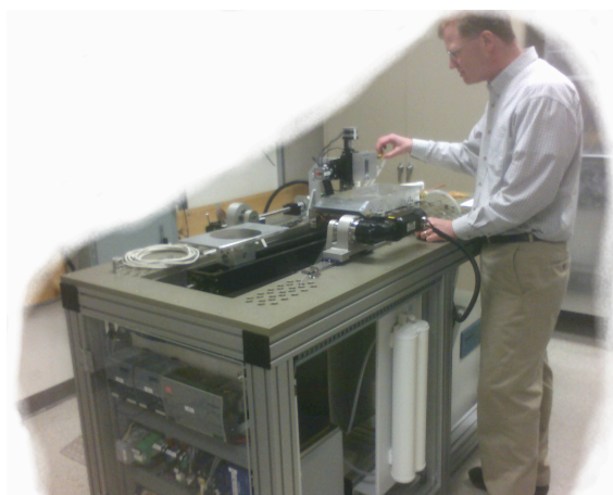
Figure 1: The monolayer nanoparticle coater
