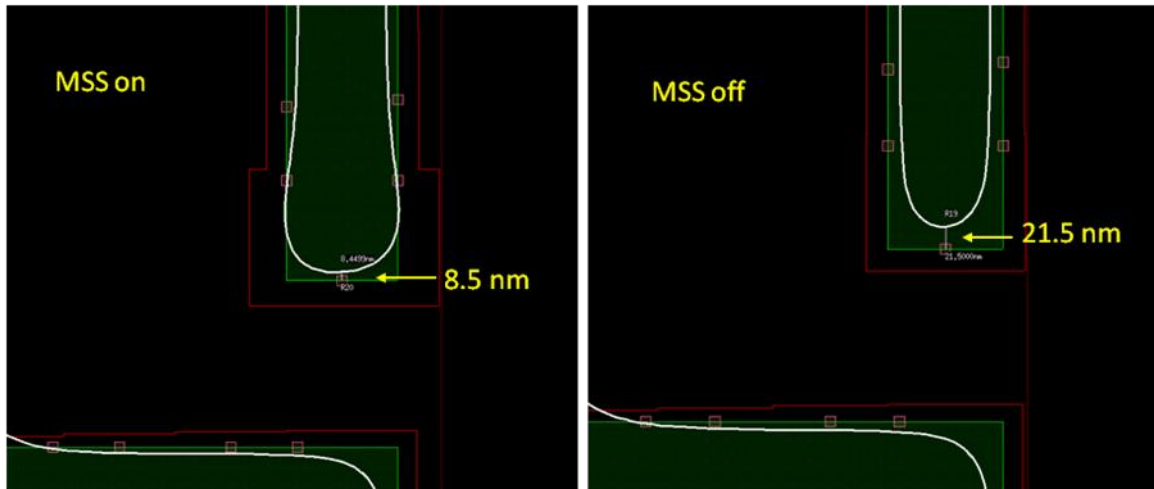
Fig. 1. Comparison of the MBOPC results with and without MSS after first iteration. The contours at line-end are significantly improved with MSS turned on.
