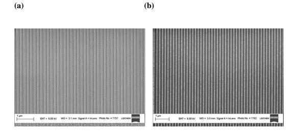
Figure 1. Top-down FE-SEM images for (a) SSQ replica of the master  $SiO_2$  mold and (b) PMMA imprint from the SSQ replica. Uniform PMMA imprints with line width approximately 30 nm from SSQ replica with trench width of 30 nm, indicate that the secondary SSQ mold can create high quality replica from  $SiO_2$  master mold and can be used as a daughter mold to generate polymeric imprint with high pattern fidelity over large area.
