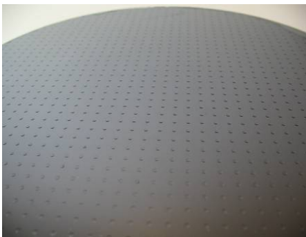
Figure 3: Photograph of an array of microlenses (diameter of lenses: 1 mm, height of lenses: 500 µm) imprinted with working stamp on 200 mm glass wafers
