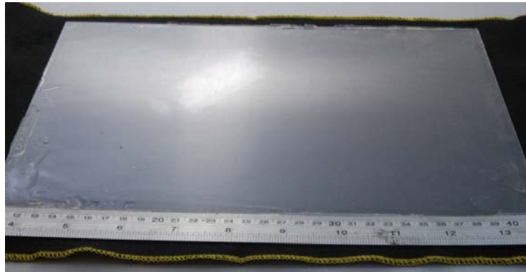
Fig. 2. The fabricated large-size (320mm × 240mm × 0.8 mm) PMMA light guide plate with dots patterns.
