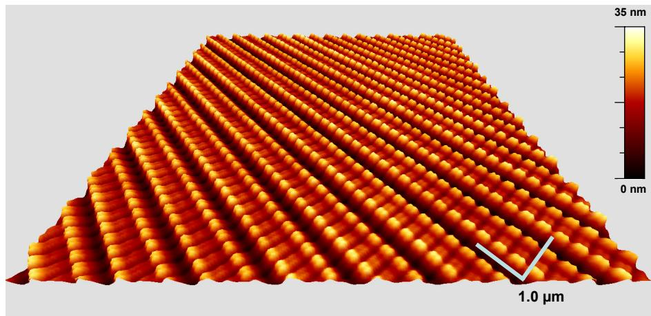
**Figure:** 2D periodic patterns generated by double exposure of the plasma deposited polymer film.
