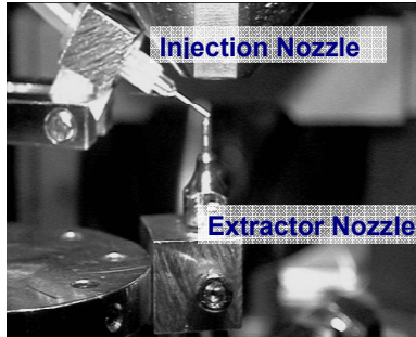
Fig.1. GIS injection nozzle and vertically mounted extractor nozzle in the system vacuum chamber of the scanning electron microscope
