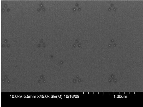
Figure 2. SEM of nanodot trimers for the binding of triangular DNA origami.
