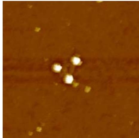
Figure 4. Dry AFM image of DNA origami on nanodot trimers. (The origami structure remains intact after drying.). Image size: 900 nm.
