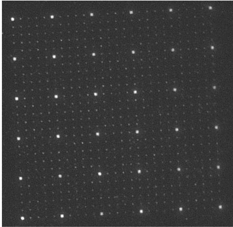
Figure 1. EPI-fluorescence image of the nanopatterned dots functionalized with a Cy3 labeled dsDNA: excitation 550nm , emission 568nm. Every fifth sub-50nm dot, a 1mm register dot is clearly visible, and brighter in the fluorescence image. Exposure time: 300ms.
