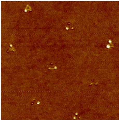
Figure 3. Liquid AFM image of DNA origami selectively bound to nanodot trimers. Image size: 1.9 $\mu$ m.
