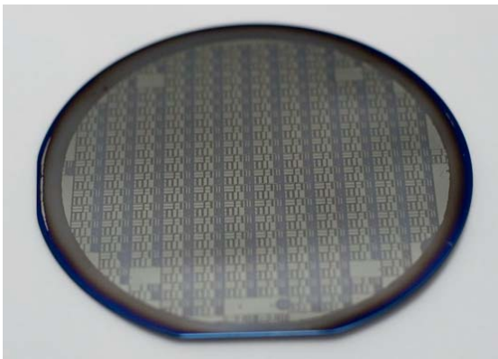
Fig 4. Post-CMP 4'' acceptor wafer with Ge (100) crystal islands on top of SiO 2 .
