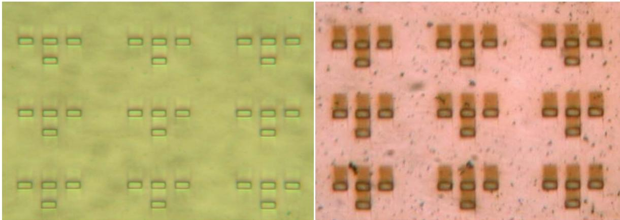
**Figure 2:** Optical microscope images of the retroreflectors before and after the enzymatic reaction: the enzyme product accumulates only in the shadowed regions where antibodies are not damaged by the ion beam.
