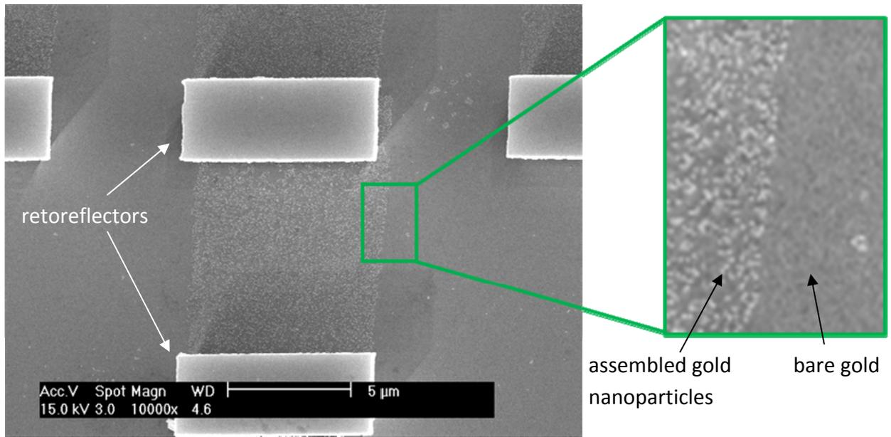
**Figure 1:** Scanning electron micrograph of gold nanoparticles assembling only in the regions that were shadowed by the retroreflector structures during the ion beam exposure. The zoomed-in image shows the high spatial resolution of the patterning step.
