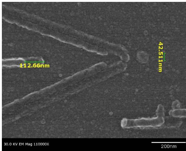
Figure 3: Aluminum-aluminum oxide single electron transistor fabricated on the silicon substrate, connected to the CMOS inverter
