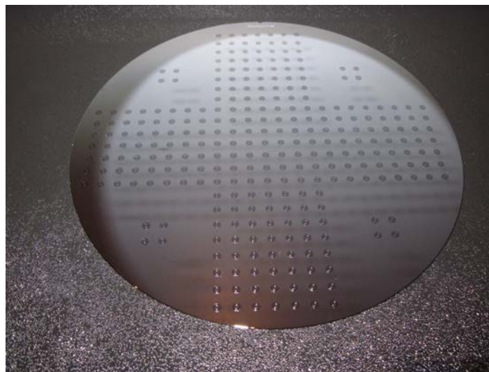
Figure 3: 200 mm master stamp with 400 replicated lenses
