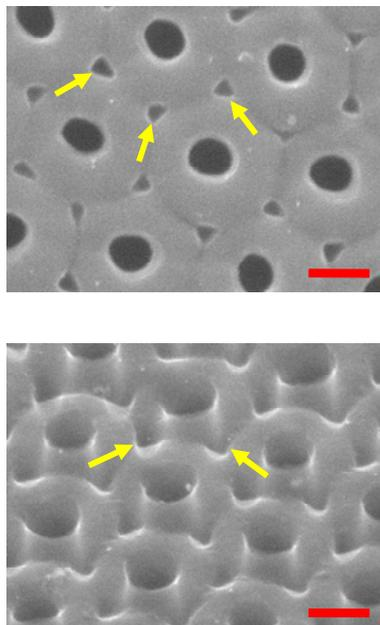
Fig. 2 SEM images of AAO: top view (upper panel) and tilted view (lower panel). Note that larger pores shown in the micrograph represent NIL mother stamp patterns replica while smaller pores indicated by yellow arrows represent newly formed pores during the course of guided anodization. Scale bar in the both images is 200nm.
