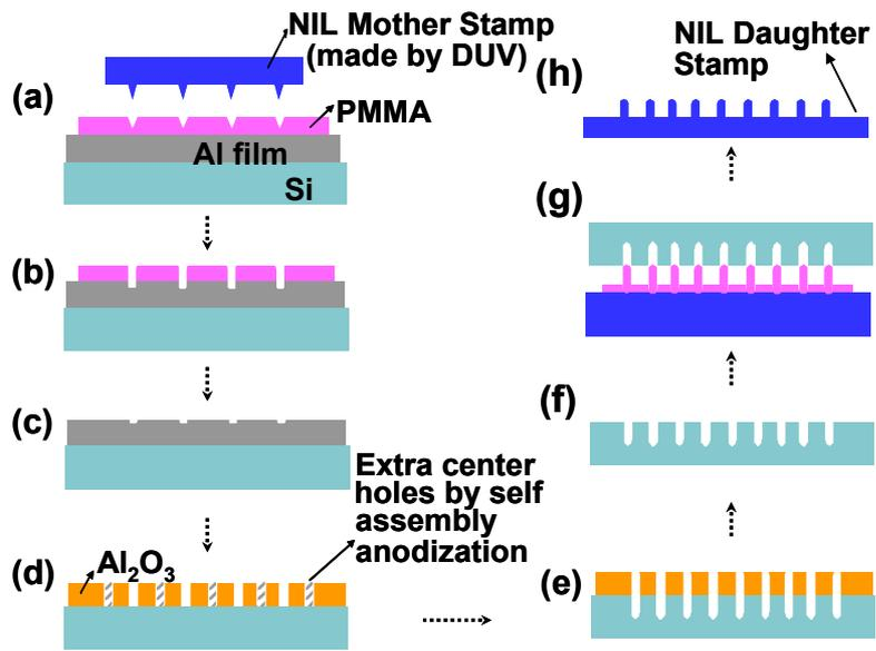
Fig. 1 Schematic daughter stamp fabrication procedures: (a) nanoimprinting on PMMA resist, (b) pattern transfer into Al film surface by RIE, (c) PMMA removal, (d) guided anodization, (e) pattern transfer into Si substrate by RIE, (f) AAO removal, (g) nanoimprinting on PMMA resist, and (h) pattern transfer into Si daughter stamp by RIE
