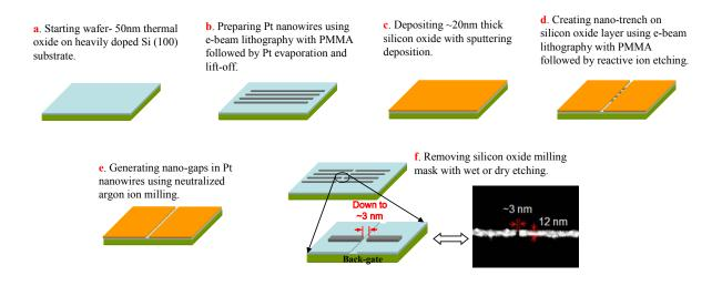
Fig 1: Fabrication process flow for down to 3nm gaps in nano-antennas.
