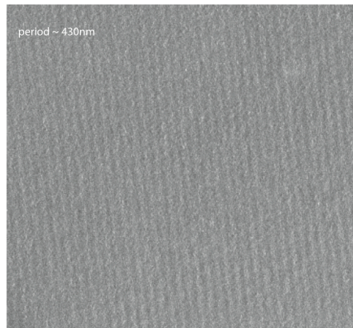
Figure 2: Scanning-electron micrograph of a grating pattern from a single-exposure with absorbance modulation. The period of the \lambda_2 standing wave was about 430nm.
